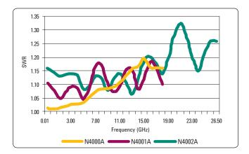
Figure 1. Characteristic SWR at 23 °C
